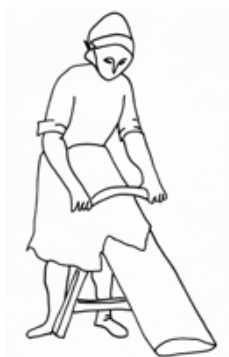
Figure 7 Fleshing beam in use with curved fleshing knife.
