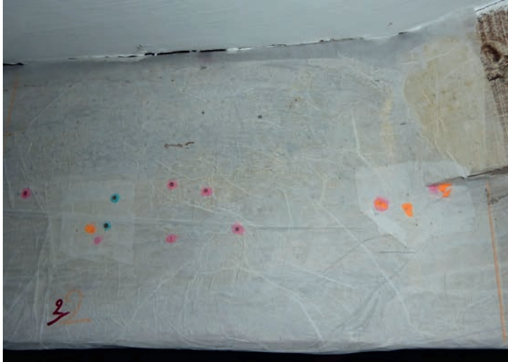
Figure 3.5 Deathwatch beetle ( Xestobium rufovillosum ) emergence through tissue paper.
